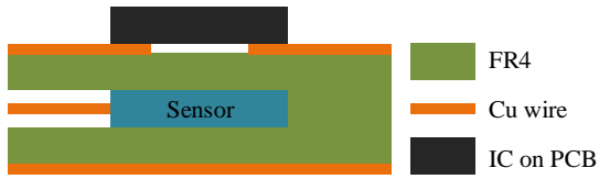
Fig. 1, Embedded sensor in a PCB
